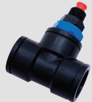
36073008002 3/4" Anti-Siphon Kit Fits all 3/4" MixRites inline to relieve pressure so chemical will not siphon out of drum or tank.
