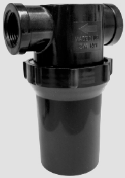
50.41.1 Female/Female 3/4" Strainer 3/4" NPT strainer with 80 micron filter cleans up any installation and improves water quality and length of service for MixRite.
